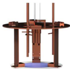
CAD model of the single-stage isolation with the experiment sitting on the bottom (blue). The springs are attached to the nylon wires at the top (white)
